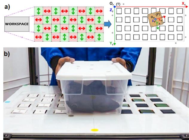
Fig. 1. (a) Voxelizing a flat workspace for omnidirectional conveyance. (b) Trackable payload placed atop the 1 \times 2 array of VERA partitions.
