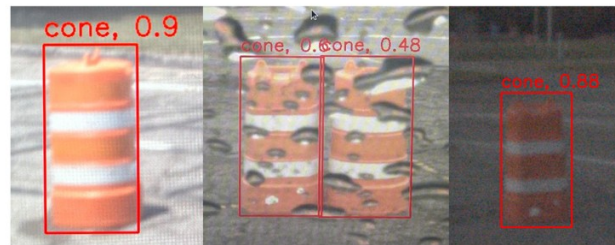
Figure 7. Sample cone detection in broad daylight, rainy weather, and after sunset
