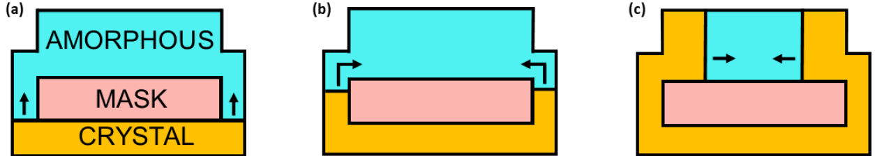
Figure 1: Masked crystal growth with a crystal substrate (orange), inert mask (pink), and deposited amorphous (blue) at successive stages of crystallization.
