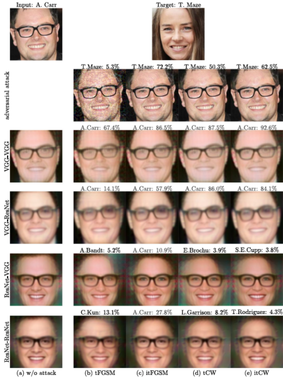
Fig. 12. Adversarial attack results without (row 2) and with (rows 3–6) the use of DFD reconstructions. Predicted identity above each image. Adversarial attack designed to fool the system into classifying A. Carr as T. Maze. DFD reconstructions show resistance to adversarial attacks, especially when reconstructing from the VGG embeddings. ResNet-based reconstructions (bottom two rows) also exhibit some characteristics of the target gender. Each column is a different attack method: (b) targeted FGSM, (c) iterative targeted FGSM, (d) targeted CW, (e) iterative targeted CW.
