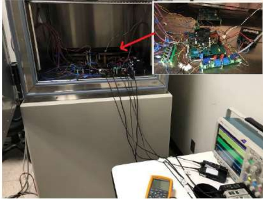
Fig. 7: Experimental setup for GaN-based H-bridge power converter with the conventional V_{DSon} measurement circuit.
