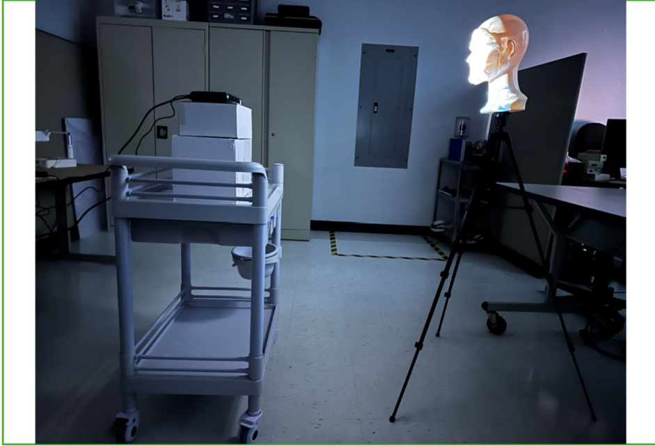
Fig. 3: Setup for projection data collection using a Miroir M600 projector, a mannequin head, and a white 3D-printed mask.
