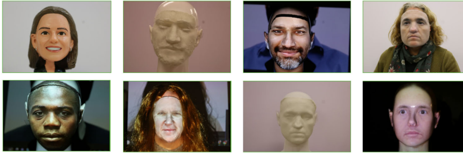
Fig. 2: Example images of PAI types developed. From Top left to right: Bobblehead, white Resin 3D mask, white resin with projection, high-quality 3D mask, a white filament with projection, hair feature on white filament with projection, white filament 3D mask, projection of face onto a 3D mannequin head.
