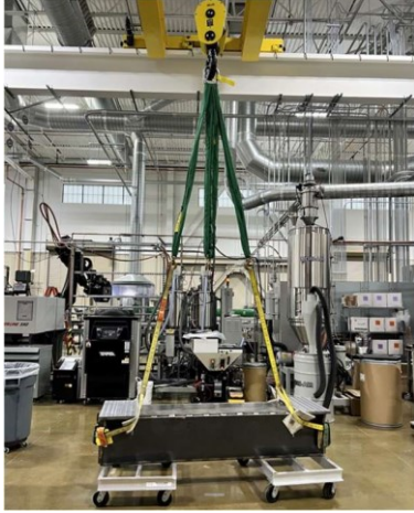
Fig. 13. Overhead crane lift of the weldment upside down for impact testing and approximate free-free boundary conditions.
