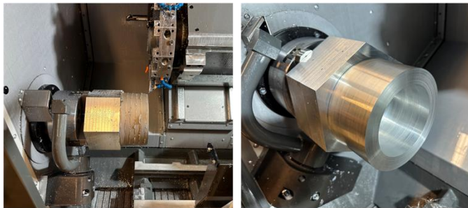
Fig. 9. (Left) preform clamped in the machine spindle prior to turning and (right) after turning operations for both the outside and inside diameters were completed.
