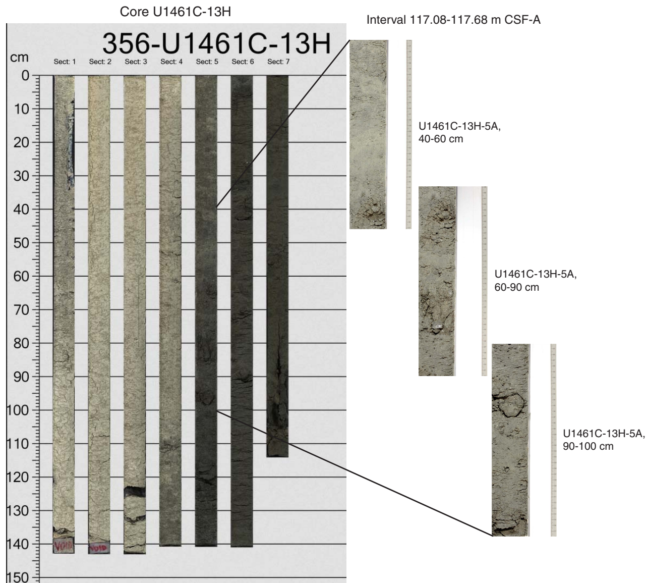
Figure F9. Boundary between Subunit IIc (unlithified cream mudstone) and Subunit IIId (olive-green packstone), characterized by common bioturbation (356-U1461C-13H-5, 40–50 cm), abundant glauconite, macrofossils (13H-5, 60–90 cm), and cementation (13H-5, 90–100 cm). Bioturbation extends from 13H-4 through the upper 10 cm of 13H-6.
