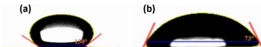
Fig. 5. Average water contact angles of: (a) PCL nanofibers, and (b) PCL/PA0.5 respectively.
