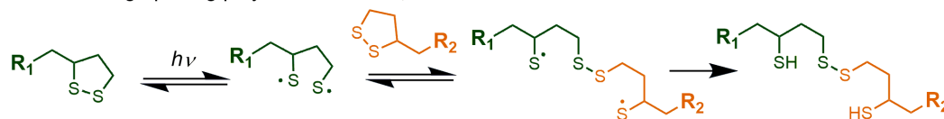
Scheme 1. Schemes of photo-chemical transformations within hydrogel networks. a) Bond breaking (i) o -nitrobenzyl ester and (ii) coumarin methyl ester; b) bond formation (i) DBCO photo-oligomerization (ii) anthracene dimerization; c) bond rearrangements (i) allyl sulfide exchange and (ii) 1,2-dithiolanes.
