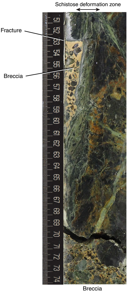
Figure F16. Cemented breccia in contact with serpentinized peridotite both at its base and along a schistose deformation zone (357-M0068A-1R-1, 50–74 cm).
