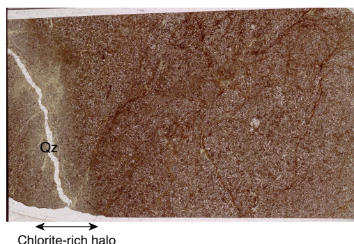
Figure F6. Background alteration of dolerite to chlorite cut by a quartz vein with a chlorite-rich alteration halo (357-M0075B-2R-1, 64–66 cm). Toward the alteration halo, thin veins change composition from iron-oxyhydroxide dominated to chlorite dominated.
