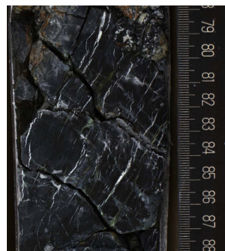
Figure F14. Series of sigmoidal to irregular isolated talc veins that form a subparallel network (357-M0068B-4R-1, 78–88 cm).
