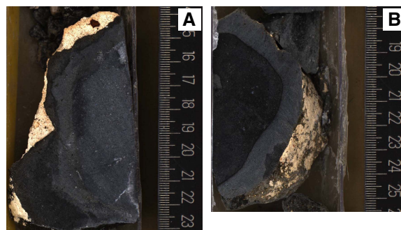
Figure F4. Vesicles lined by clay minerals (blue) and orange iron oxyhydroxides (357-M0070B-1R-1, 8–11 cm).
