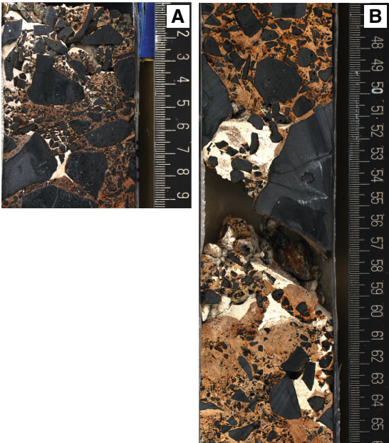
Figure F6. Sections of basalt breccia cemented by an early orange-brown matrix with voids infilled by later light tan carbonate. A. 357-M0070A-3R-1. B. 357-M0070C-1R-1.
