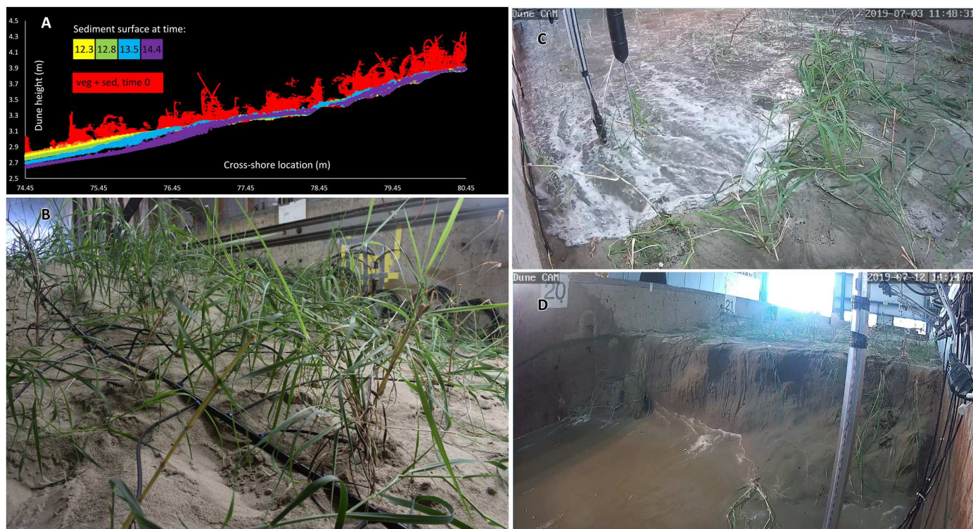
Fig. 4. Morphologic changes on VD during the extreme storm event. (A) An example of Terrestrial Laser Scanning (TLS) data for the VD profile, viewed from the cross-shore dimension (i.e., the side), at 0, 12.3, 12.8, 13.5, and 14.4 hours into the storm conditions. The red points depict both the vegetation and the sediment surface before the experiment began at 0 hours. The other colors depict the sediment surface only, between 12.3 and 14.4 hours. By 14.4 hours, an initial 0.1-m tall scarp was apparent at ~76.5 m. (B) P. amarum plants on VD before the experiment began at 0 hours. Drip line (black hose) was removed during experimentation. (C) Run-up intercepting plants on VD at 11.3 hours. The depicted sensor array included an optical sediment gauge, sediment movement sensor, ultrasonic sensor, and acoustic velocimeter. (D) A 0.79-m tall scarp on VD at 18.4 hours.
