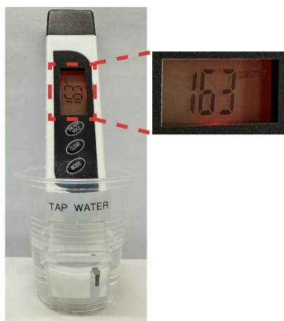
Figure 5. Samples were analyzed by immersing a conductivity meter probe into solution. Conductivity values (in units of \mu\text{S}/\text{cm} ) of salt water were larger than tap water because of the higher ion content. Higher temperatures increased conductivity for both samples because of the enhanced thermal motion.
