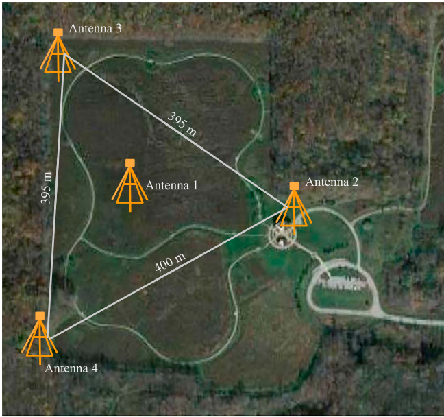
Figure 1. Aerial site map of Observatory Park with locations of each DLITE antenna indicated by orange diagrammatic antennas. DLITE arrays are composed of four dipole antennas. Due to the small number of elements in the array, the optimal configuration for the DLITE array is an equilateral triangle with one antenna at each point and a fourth in the middle. This configuration maximizes the number of unique baselines for a four-element array, which increases imaging and source tracking capabilities. In order to resolve the brightest radio objects in the sky, the three corner antennas should be separated by at least 250 m, with the optimal separation being between 350 and 500 m. The separations between the three outer antennas of DLITE Ohio are highlighted, with all separations being around 400 m based on Google Maps measurements (J. F. Helmboldt et al. 2021). Antenna 2 ( 41^{\circ}35'07''.2\text{N} 81^{\circ}04'49''.4\text{W} ) is the closest to the Observatory Park Science Center and parking lot, Antenna 3 ( 41^{\circ}35'14''.0\text{N} 81^{\circ}05'03''.9\text{W} ) is located in the far northwestern corner of the park, Antenna 4 ( 41^{\circ}35'01''.3\text{N} 81^{\circ}05'04''.9\text{W} ) is located in the far southwestern corner of the park, and Antenna 1 ( 41^{\circ}35'08''.0\text{N} 81^{\circ}04'59''.4\text{W} ) is centrally located in the park. Each antenna location has a unique radio-frequency interference (RFI) environment, with Antenna 2 seeing on average more RFI than the other three antennas, likely due to a transformer box close by. Observatory Park is well shielded on all sides from RFI due to the mature forest surrounding the telescope site (T. Tamir 1967).
