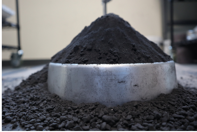
Fig. 1. Example of a fine-coarse mixture of asteroid regolith simulant. This sample is composed of mm-sized grains mixed with a 25% fine-fraction. The picture was taken during an AOR measurement.
