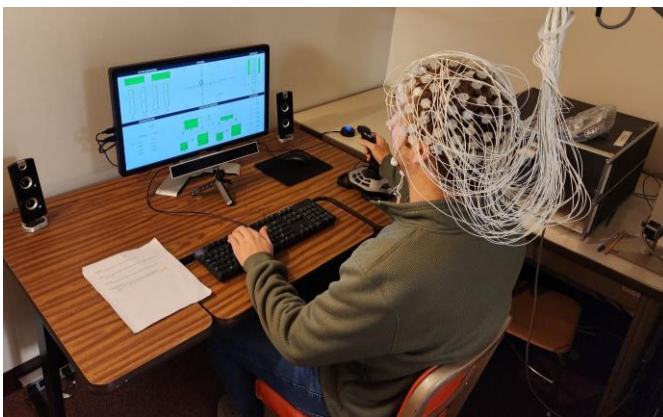
Figure 1. A person interacts with the adaptive OpenMATB scenario while monitored using both the electroencephalography sensor net and the eye tracker. Actual participants experienced only one sensor type.
