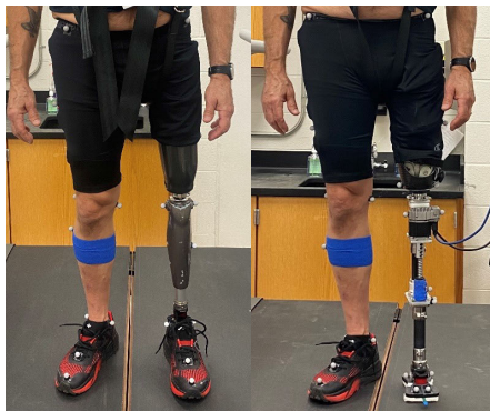
FIGURE 9. Subject 1 wearing his HK (left) and the developed LAP (right) attached with reflective markers.
