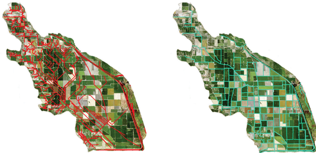
FIGURE 16 Elevation-derived flowlines (red lines) and flowlines from NHD (cyan lines) in Long Lake-Sutter Basin watershed, CA.
