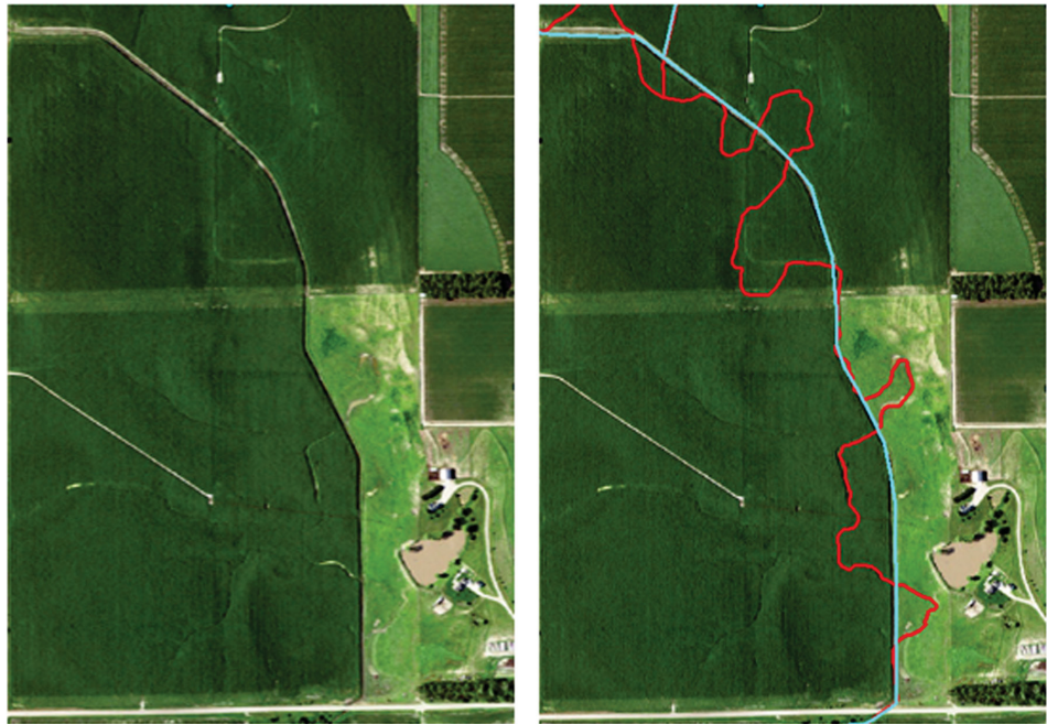
FIGURE 2 An example of NHD update caused by terrain surface changes. An artificial ditch was constructed after NHD generated (left). In the right image, the red line represents the original NHD flowline, while the cyan line is the corrected NHD flowline.
