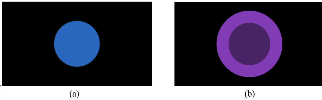
Fig. 6. Projected optical masks during the PinPAM process of printing a single pillar. All masks are grayscale in the actual implementation of the PinPAM process; the curing mask is shown in blue and inhibition mask is shown in purple only for visualization clarity. (a) Curing mask of blue light circle. (460 nm, 8 mW/cm 2 , diameter measured on the build plane: 4.5 mm). (b) Inhibition mask with a UV circle (365 nm, overlapping with the blue light circle in (a)) and a ring (circumferential to the curing circle). The UV light intensity is proportional to the grayscale of UV mask, with the grayscale 255 providing a maximal intensity of 12 mW/cm 2 . Brighter color indicates greater inhibition intensity. (For interpretation of the references to color in this figure legend, the reader is referred to the Web version of this article.)
