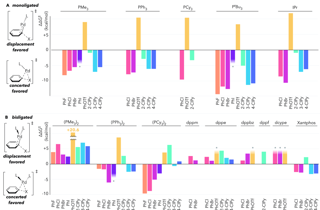
Figure 2. Difference in free energies of activation for displacement versus concerted transition structures for (A) monoligated Pd and (B) bisligated Pd.
