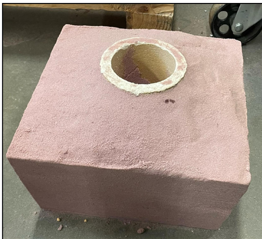
Figure 7. Insulated mold made with an insulation sleeve and no-bake sand used for thermal analysis.
