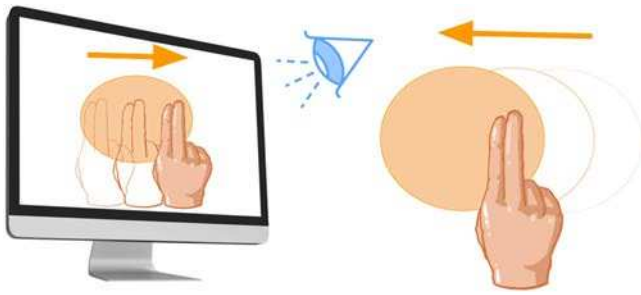
Fig. 1. Passive touch method. Passive presentation of an active task: A passive user observes video of active hand motion while a 2D robotic platform recreates the relative motion between the hand and object.
