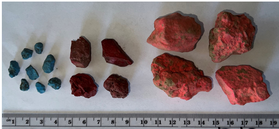
Figure 2. Examples of small (left, blue), medium (middle, red), and large (right, pink) experimental particles used in particle drop experiments in summer 2021 and spring 2022. Ruler units are in centimeters.
