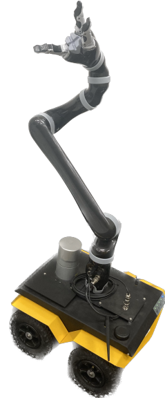
FIGURE 1. KINOVA GEN2 ROBOTIC ARM MOUNTED ON JACKAL GROUND VEHICLE.
