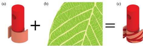
Figure 5: Biologically inspired functionally graded materials applied to deployable anchor: anchor model (a); leaf, as inspiration (b); pattern applied onto awn (c).
