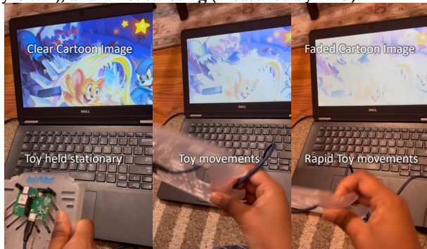
Figure 7: Keeping the toy stationary leads to a clear enjoyable cartoon image on the screen. Movements of the toy starts to wash-out the image.
