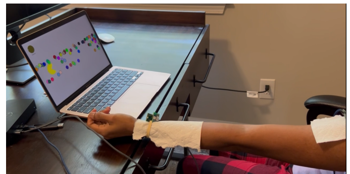
Figure 5: Arm bending at the elbow being used as input to play a computer game where a Pac-Man figure eats candy on the screen by moving back and forth.
