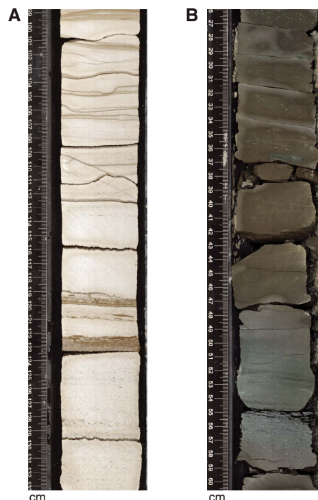
Figure F27. Cores rated strong and brittle in strength. Brittle fractures, abundant natural faults, and some drilling-induced biscuits are present, but sections are more coherent. A. Calcareous pelagic sediment (Section U1480G-61R-3). B. Clay-rich hemipelagic sediment. Fissile fractures are abundantly observed (Section U1480G-58R-1).
