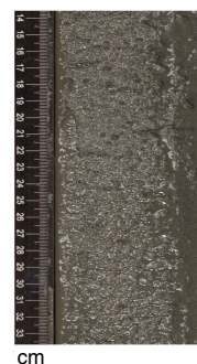
Figure F25. Soupy section in the sediment caused by drilling disturbance in which the primary structure is destroyed (Section U1480F-13F-3). Note the presence of water even after efforts to drain the core.
