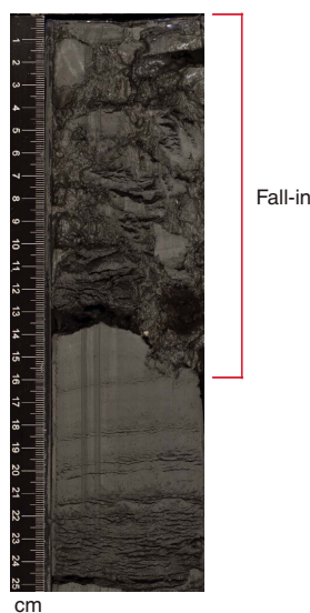
Figure F24. Fall-in at top of core (Section U1480F-12F-1). Fall-in was present at the top of many cores and was given a drilling disturbance intensity rating of destroyed.
