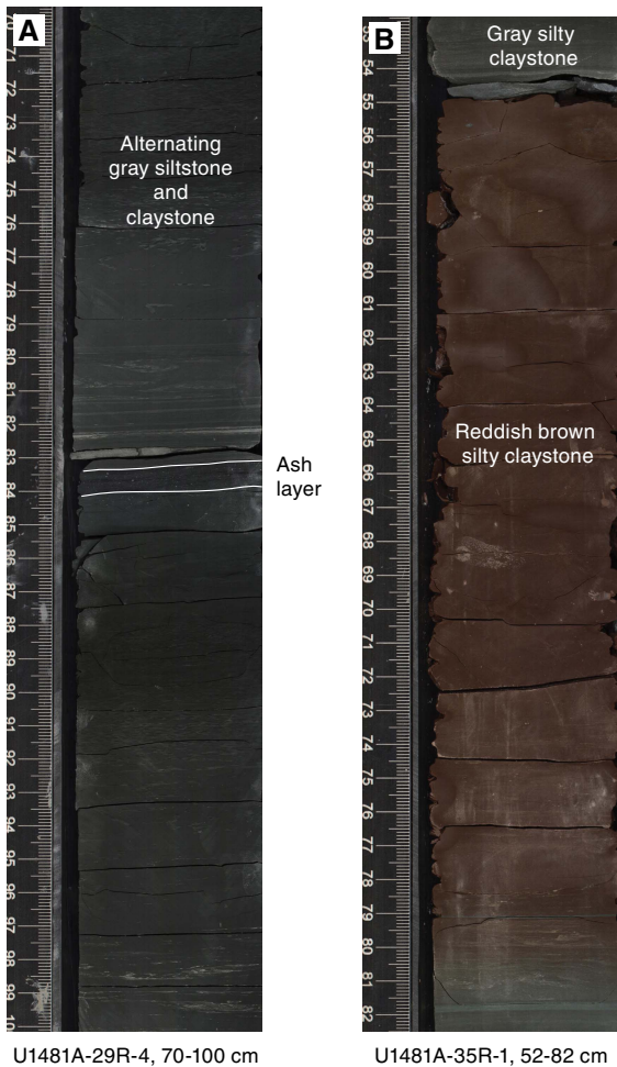
Figure F6. A. Alternating gray siltstone and claystone from Unit III (equivalent to Subunit IIIA at Site U1480). Note the 1 cm thick ash layer (bound by white lines) (1406.88–1407.18 mbsf). B. Minor reddish brown silty claystone and gray silty claystone from Unit III (1461.42–1461.72 mbsf).
