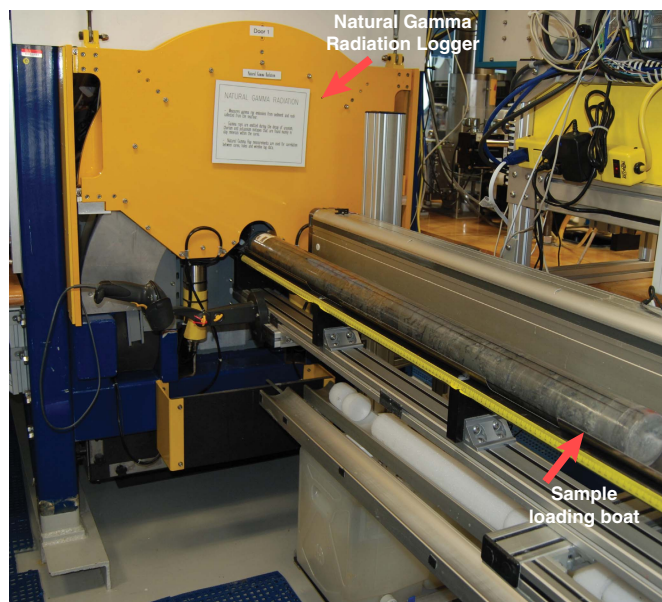
Figure F14. NGRL for whole-round cores, Expedition 363. The NGRL conducts 8 measurements at a time in 2 positions, resulting in 16 measurements per core when measuring at both positions.
