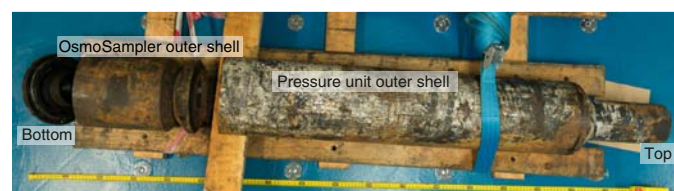
Figure F8. Photo of GeniusPlug after recovery. P = pressure.
