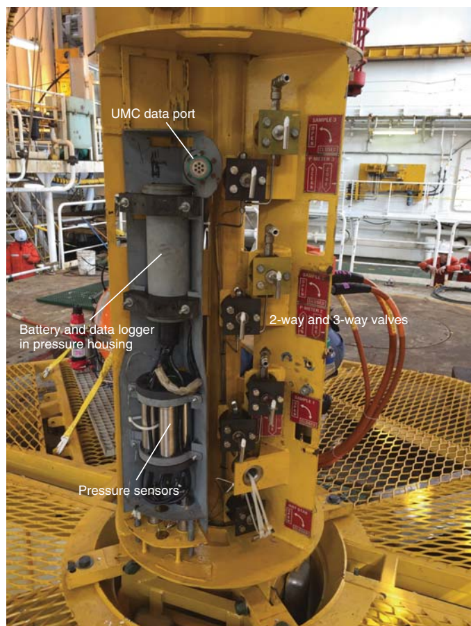
Figure F14. Bay 1 of LTBMS head, holding the PSU with four high-precision quartz pressure sensors (Paroscientific, Inc.) and two-way and three-way valves. Note cylindrical pressure housing with data logger and PPC unit. See text.
