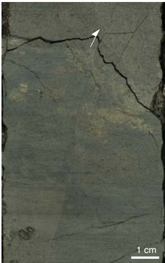
Figure F30. Split core image of a reversed fault (365-C0010E-3R-4, 13–23 cm; ~375.6 mbsf). Arrow = sense of slip.
