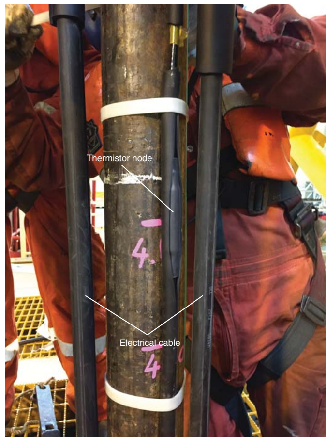
Figure F15. Spacing of centralizers, tie wraps, and steel bands used to secure cables to 3½ inch tubing, Hole C0010A. FWD = forward.
