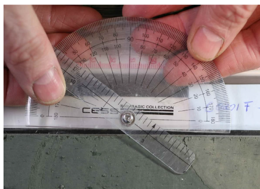
Figure F9. Protractor used to measure apparent dips, trends, plunges, and rakes on planar and linear features in a split core, Expedition 366.
