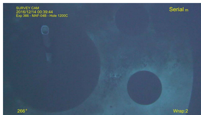
Figure F2. ROV platform, Hole 1200C. The tube that extends from the hole is a schedule 80 PVC tube that was deployed in 2009 (Figure F3).
