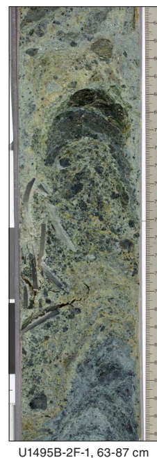
Figure F32. Drilling disturbance-induced structures (366-U1495B-2F-1, 63–87 cm) including up-arching caused by flow-in of darker serpentinite mud matrix. Core photo also shows a cluster of broken elongate pieces of damaged plastic core liner that have flowed-in from lower in the core.
