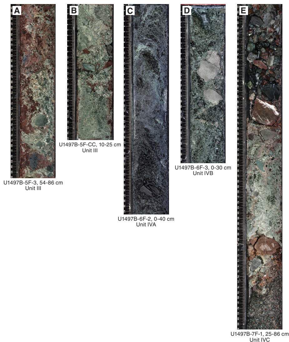
Figure F9. Major lithologies, Hole U1497B. A. Highly deformed sedimentary and volcanic rocks (Unit III). Light clasts are volcanic rocks. B. Mixing of red sedimentary and white volcanic material (Unit III). C. Serpentinite mud and clasts deformed by drilling (Subunit IVA). D. Clast-rich matrix with both serpentinized ultramafic and metavolcanic rock (Subunit IVB). E. Sedimentary and volcanic rocks (Subunit IVC).
