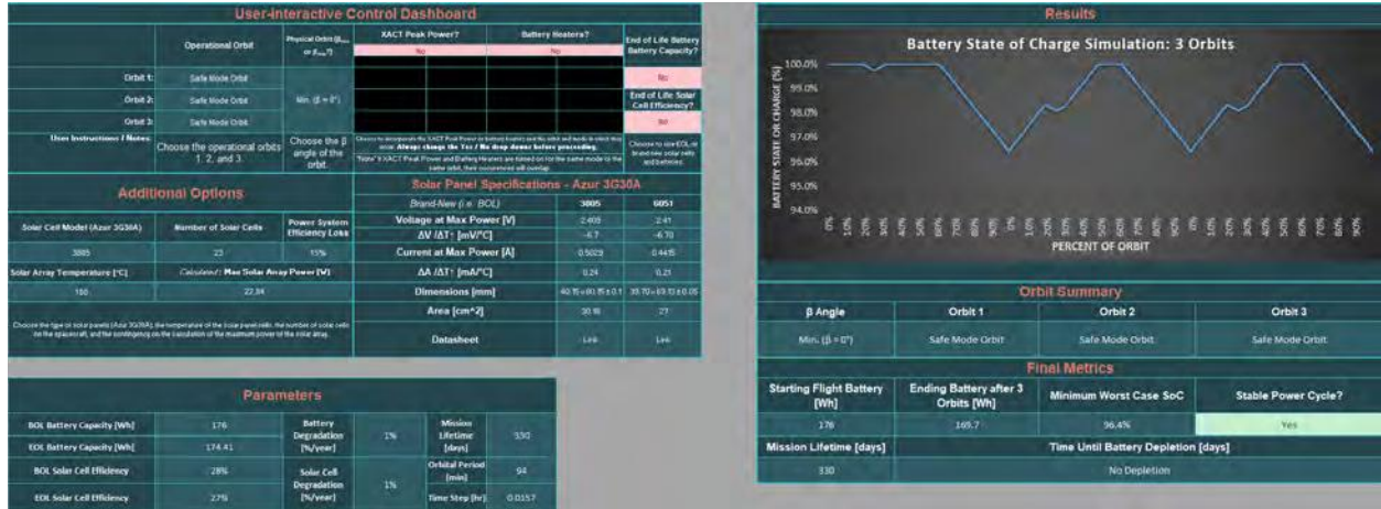
Fig. 18 A screenshot from the SWARM-EX power budget illustrating its capability to simulate the battery SoC for three orbital timelines (three Safe Mode orbits at \beta = \beta_{min} are shown) of the user's choosing, allow the input of various parameters, and identify the stability of the spacecraft power state.
