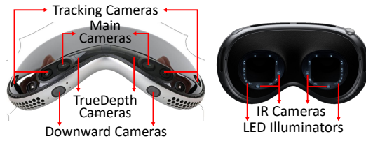
Figure 2: Cameras on Apple Vision Pro.
