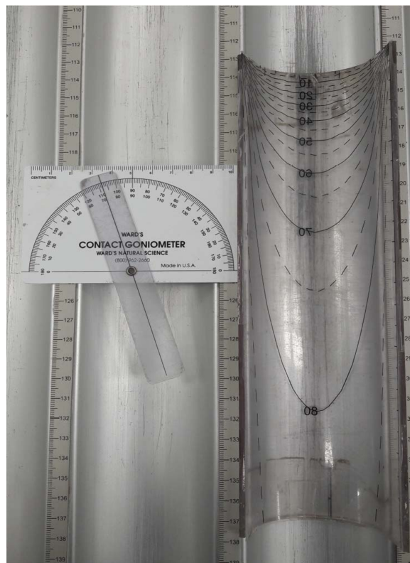
Figure F18. Goniometer and plastic protractor template used to measure dip and dip direction of structures, Expeditions 367 and 368.
