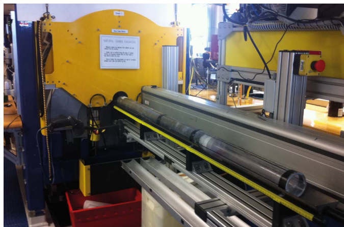
Figure F26. NGR for whole-round cores (conducts 8 measurements at a time in 2 positions, resulting in 16 measurements per core), Expedition 367 and 368. During Expedition 367, scintillation Detector 7 was deficient, so only 14 measurements per core were performed.
