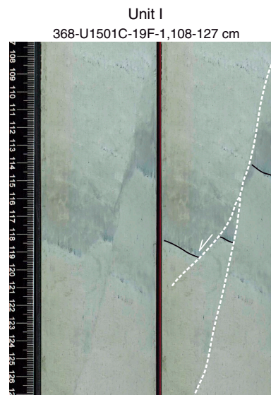
Figure F26. Deformation structures, Unit I. Normal fault affecting nannofossil oozes (368-U1501C-19F-1, 108–127 cm).
