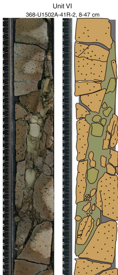
Figure F38. Strongly fractured and fragmented basalt filled by fine-grained unconsolidated greenish rock, top of Unit VI.
