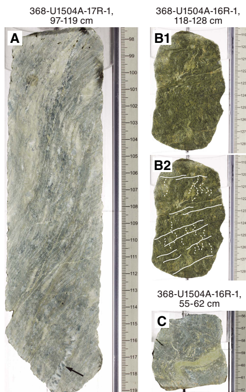
Figure F22. Ductile deformation structures in epidote-chlorite schists in Sub-unit IIIA, Hole U1504A. A. Steep (~75°) widely anastomosing foliation in a quartz-rich variety of the rock. Arrow = extensively stretched veined clast of chlorite-epidote granofels, oriented parallel to the foliation. B. Tight foliation affected by crenulation cleavage in quartz-poor variety of the rock (top: core photo; bottom: interpretation). C. Folded epidote vein.
