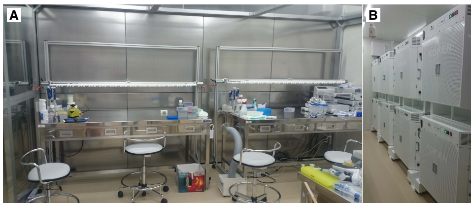
Figure F23. Super-clean room at KCC. A. Clean working area for sample processing. B. Floor KOACH Ez units for super-clean room.
