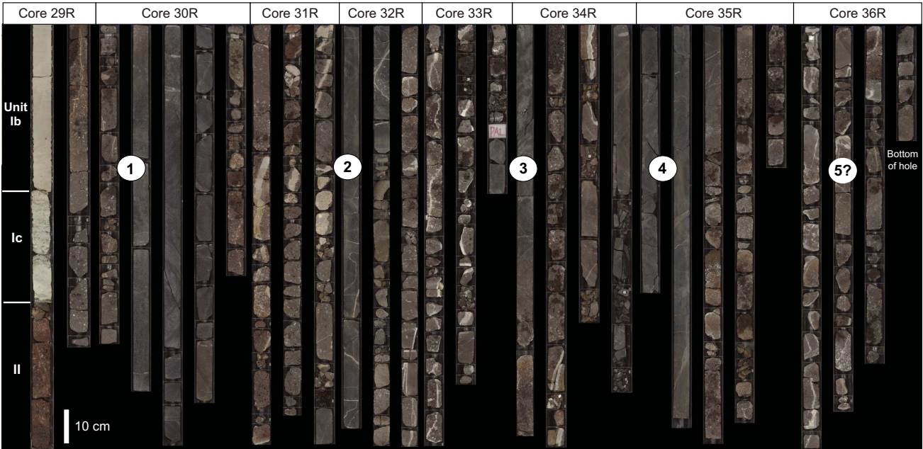
Figure F11. Repeated sequences (4 or 5) of alternating reddish brown microcrystalline amygdaloidal basalt and massive fine-grained dark gray basalt from Unit II, Site U1506. Sequences are numbered on fine-grained dark gray facies that represent the center of the sequence, whereas sequence boundaries are not clearly visible.
