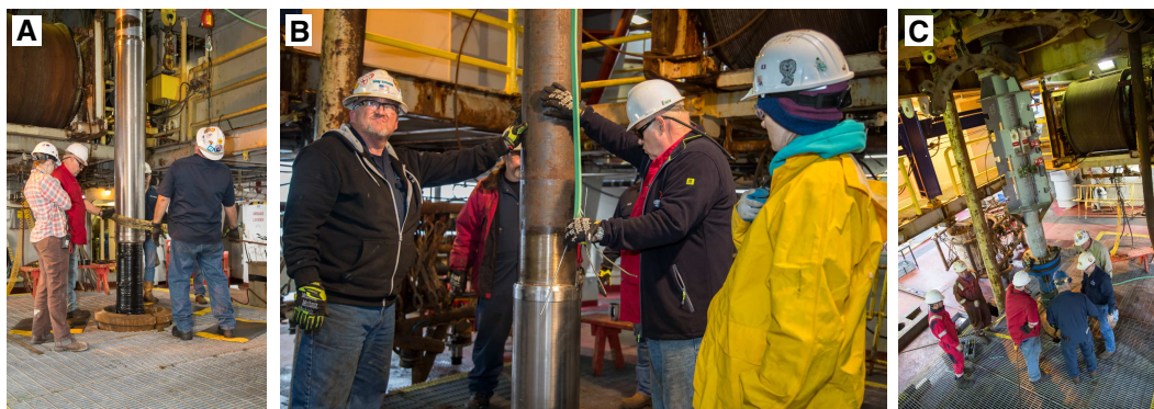
Figure F44. Pressure sensing components, Hole U1519B. A. Pressure monitoring screen. B. Hydraulic lines in umbilical (green) being attached to pressure monitoring screen on exterior of ACORK casing. C. Pressure valves and external sampling ports on ACORK wellhead.
