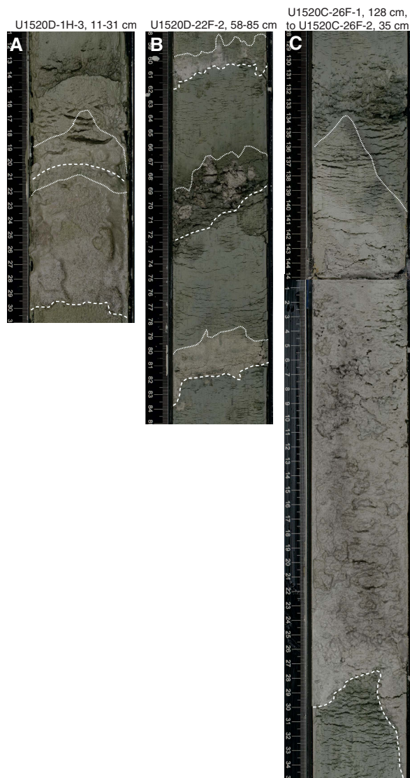
Figure F32. Examples of tephra layers in Units I-III, Holes U1520C and U1520D. Dashed lines = base, dotted lines = presumed top of original ash layers.
