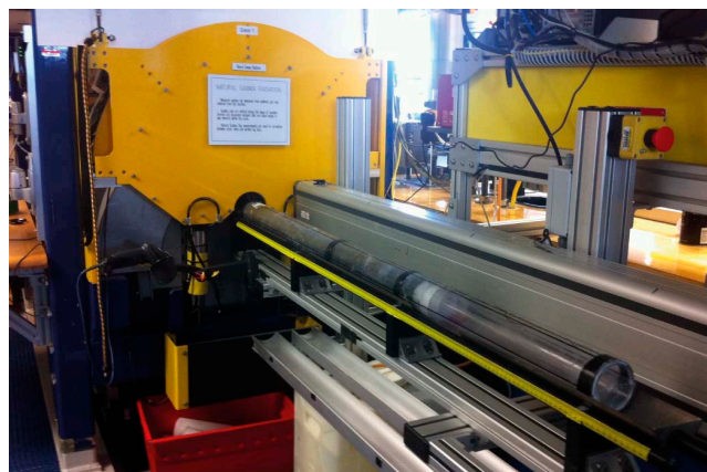
Figure F18. Shipboard station for measuring thermal conductivity on whole-round and section-half cores.
