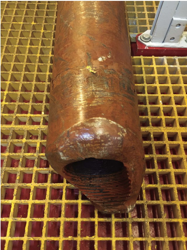
Figure F6. Damaged bit sub recovered from the end of the drill string pulled out of Hole U1527B. Bit sub was damaged beyond repair by wearing during drilling in casing after the pilot bit had failed. (Credit: Tobias W. Höfig, IODP JRSO)
